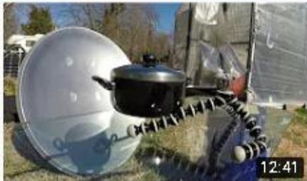
Parabolic Satellite Dish Solar Cooker
