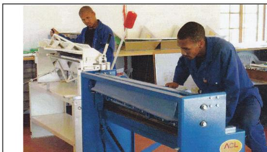
The cooker production requires a guillotine shear (left), a sheet metal bender (right), a circular saw and a hand-drill.
