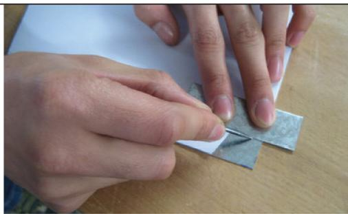
True size paper templates of all metal cooker parts with all particulars make measuring almost unnecessary and facilitate production.
