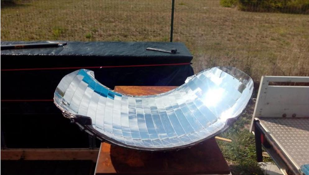
The secondary mirror is made of aluminium foil.
