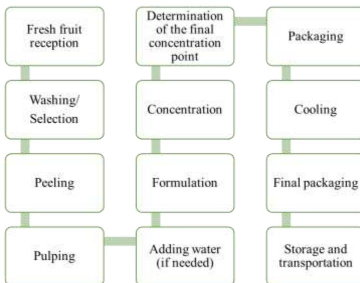
**Figure 7.** Flowchart of the candy manufacturing process.
