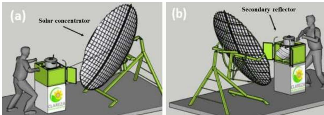
**Figure 1.** Perspective of the heating system with detail for the reflective material of the solar concentrator (a) and the secondary reflector (b).
