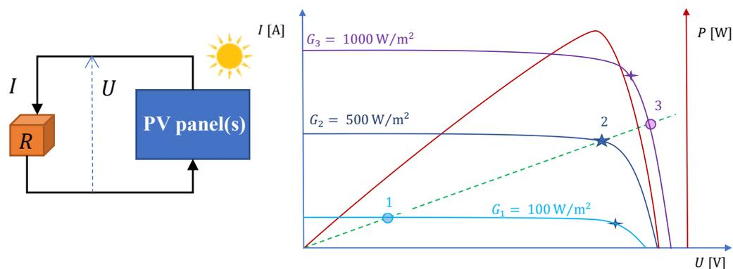
Figure 1.- Relations between voltage  $U$  and intensity  $I$  of a PV panel in good condition for three irradiances, the curve for a resistance  $R$ , and the power  $P$  delivered for only  $G_2$  and  $R$  for MPP at  $G_2$ .
