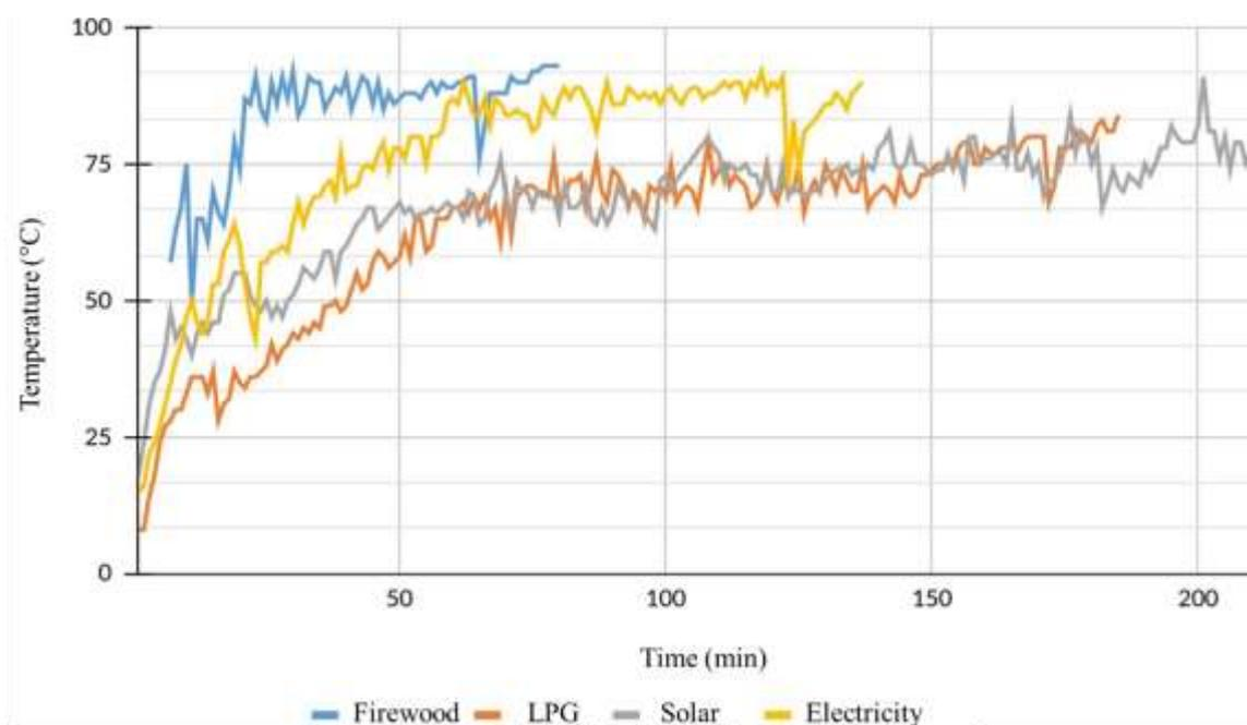
**Figure 9.** Temperature profile over the total cooking time for each process, with readings every 60s.
