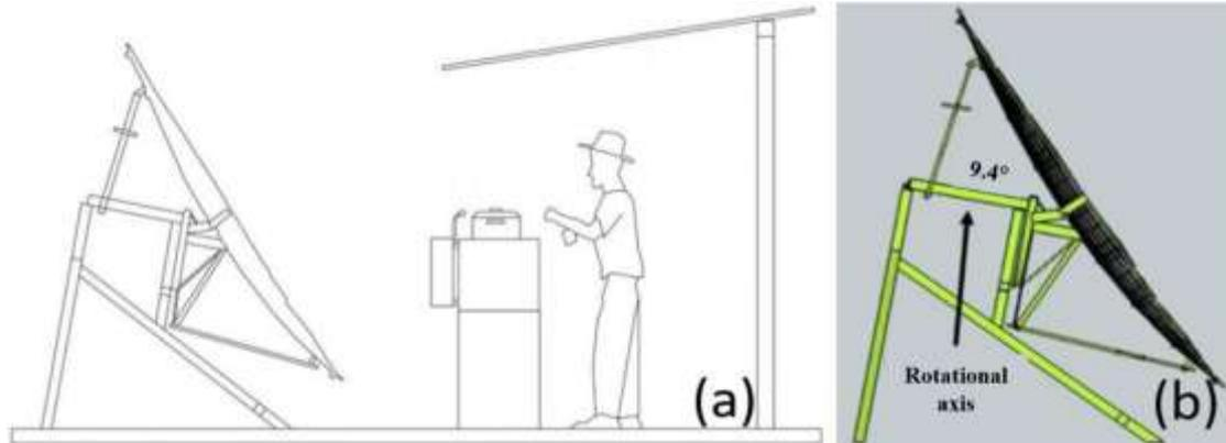
**Figure 2.** Side view of the solar concentrator with cover (a) and rotation axis adjusted to the latitude of Paulo Afonso - Brazil (b).
