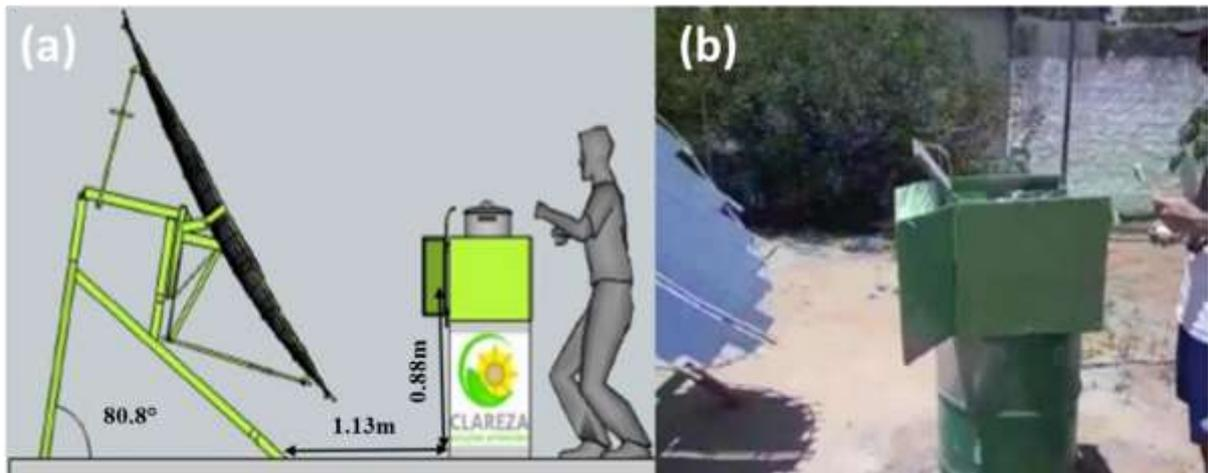
**Figure 8.** Side view of the project (a); side view of the prototype built in this work (b).
