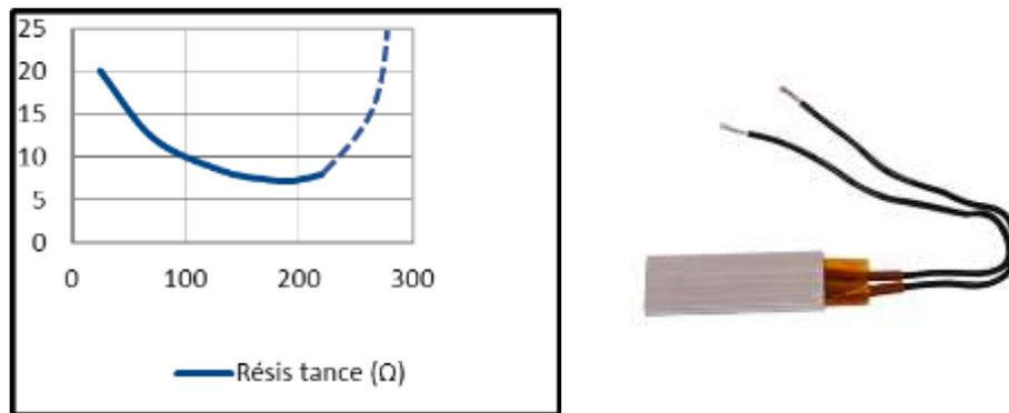
Figure 2.- Left) Example of the variation of the resistance  $R$  of a PTC element as a function of its temperature, obtained with the test bench herewith proposed. Right) example of a PTC heater element with a rated power of 35 to 80 W.
