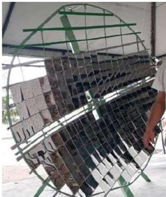
**Figure 4.** The final manufacturing process of the solar concentrator: installation of reflective material.
